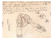
Cross-rolling process sketch of Max Mannesmann, pre 1885
